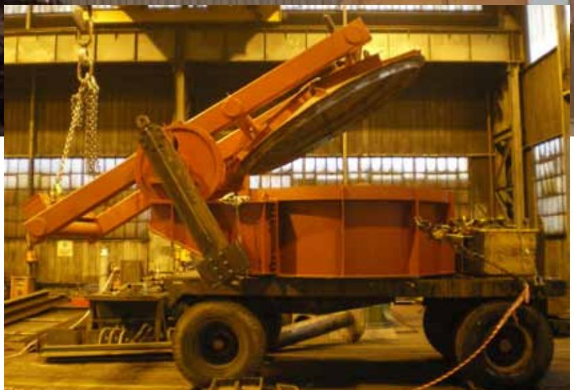
Stack Cap Fabricated in Evraz Highveld Workshops
